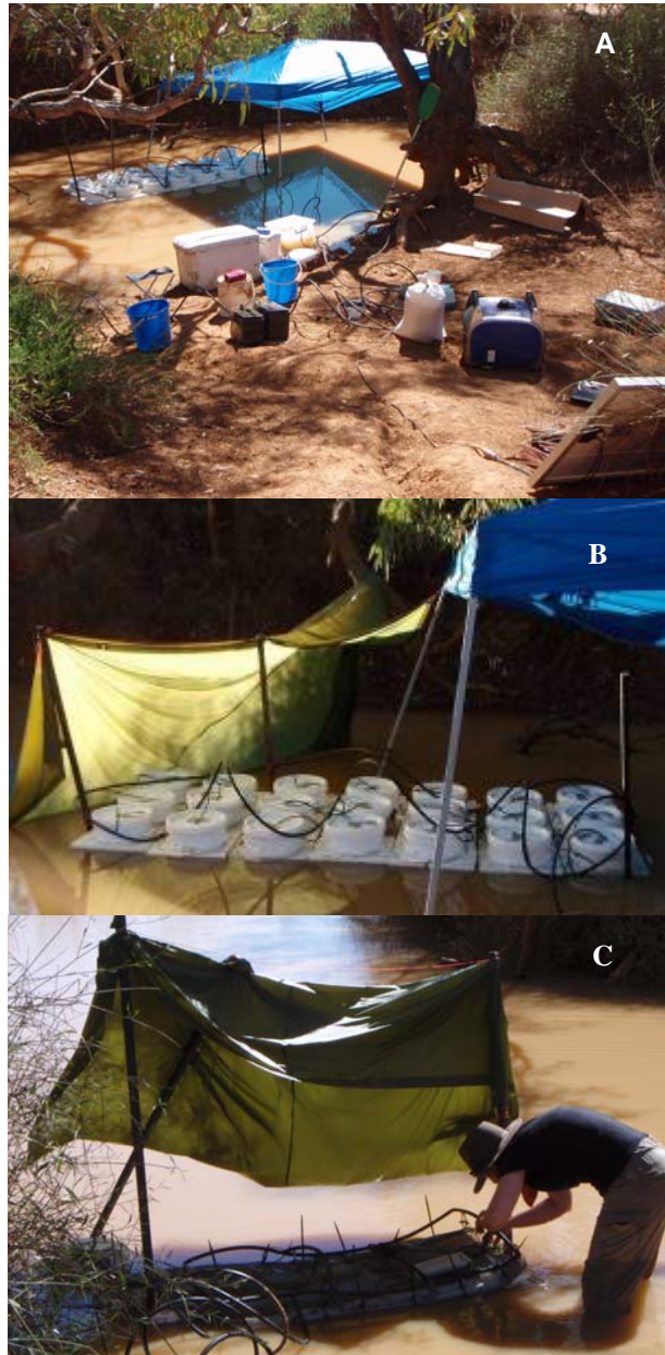
Figure 17. A) Makeshift field laboratory for salinity trials allowing three trials of six salinity treatment levels. Buckets (20L) for larger fish species and (B) 1L containers for smaller species (C) floating on polystyrene pontoons partially immersed in water at Algebuckina Waterhole and aerated using a solar powered pump.
