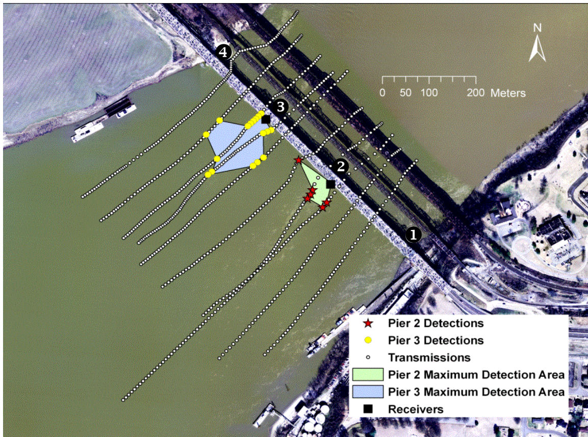
Figure 2. Locations of a submerged acoustic tag during transmissions, locations of the tag when two VR2W submersed ultrasonic receivers recorded a tag reception, and maximum reception area of each receiver during high river stage tests on 5 August 2008 at the Interstate 55 Bridge in Memphis, Tennessee. The spacing of bridge piers 1 through 4 is indicated. The main channel runs between piers 1 and 2. Photo taken at an unknown date at a high river stage.
