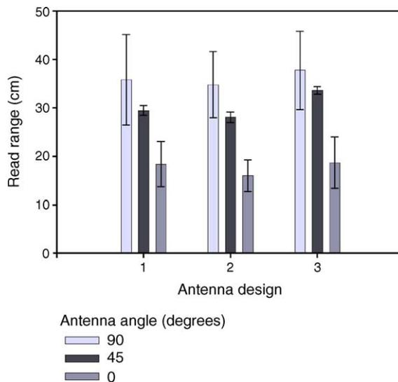
Fig. 2. 2003 antenna design comparison several wraps of: (1) 14 gauge ribbon cable to fit inside of 1 inch PVC pipe; (2) 12 gauge wire loosely gathered together to fit inside of 1 inch PVC pipe; and (3) 12 gauge wire laid side-by-side (non-overlapping) to lie flat in sheet PVC. Read range was measured at eight equally spaced intervals around the antenna at 0°, 45° and 90° (in air) for the three models. Mean read range and standard deviation (error bars) are displayed.
