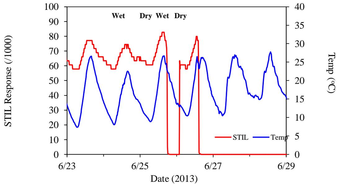
**Figure 2:** Stream temperature and wet/dry status within the thalweg of Sangre de Cristo Creek near Fort Garland, Colorado.
