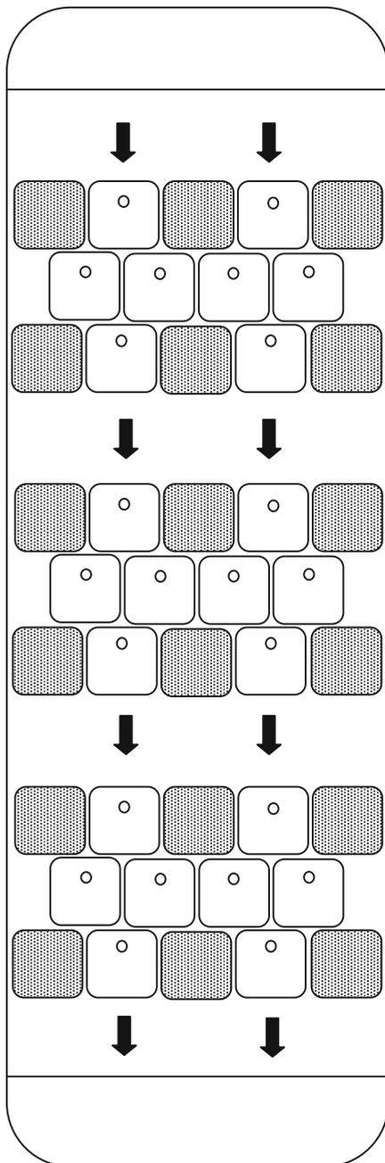
**Fig. 2** Grid-like arrangement of incubation cells (white) and non-incubation cells (shaded) used to test the affects of fine sediment on survival of eggs to larval emergence robust redhorse. Circles represent standpipes used to monitor dissolved oxygen concentrations, which are upstream of egg pockets. Arrows denote direction of water flow
