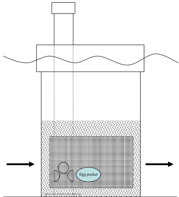
**Fig. 1** Diagram of incubation cell (15.5 L square bucket) used to house gravel treatments and incubate robust redhorse eggs and larvae. The grid is the 15×10 cm fiberglass mesh screen and the small dots represent the gravel mixture. The standpipe (3.2 cm diameter, 40 cm long) with holes (1.9 cm diameter) allowed dissolved oxygen concentrations to be monitored at depth of the egg pocket. Arrows denote direction of water flow
